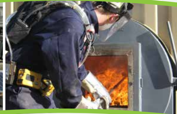
Small-scale incinerators with secondary burn chambers were evaluated for their potential to reduce environmental and human health risks from the burning of contingency base solid waste.
