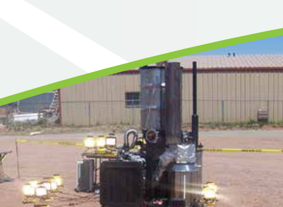
A small-scale WTE system powers lights using wood chips and refuse-derived fuel, representative of solid waste generated in theater.
