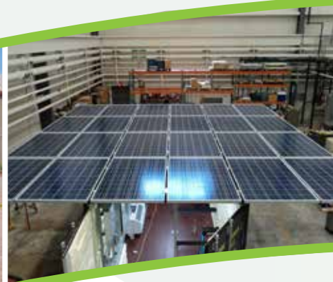
The Renewable Energy Suite integrates biomass, PV, and batteries to provide mobile power at remote sites. Mounting the PV arrays directly on the system's shipping containers helps to enhance mobility for in-theater applications.
