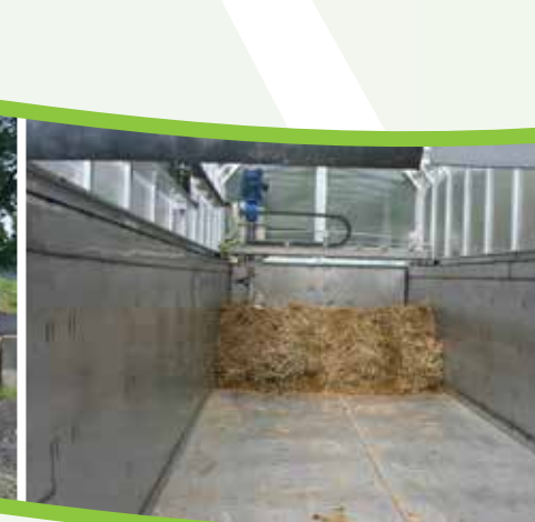
An inclined auger mixes and aerates organic waste to achieve conversion to compost within three weeks, indexing the material to the back of the container for easy removal and use.
