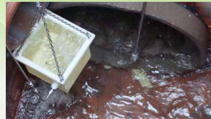
Wastewater samples were taken from an outfall at RFAAP's acid area for a batch-process demonstration of CCIX that resulted in 97% nitrate removal.
