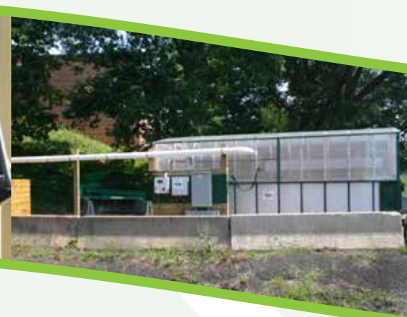
In-vessel composting systems, such as this unit transitioned to JBM-HH, enable rapid conversion of food and other organic waste to compost in a more compact footprint as compared to traditional methods, such as windrows and aerated static piles.
