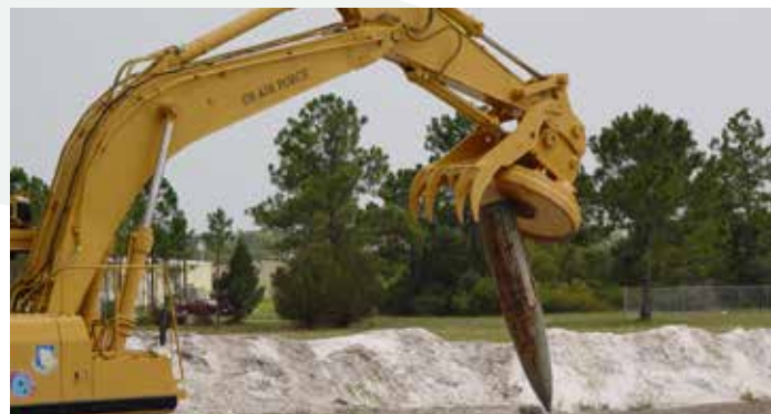
The Magnetic Unexploded Ordnance Recovery System was used to simulate magnetic recovery of munitions during an NDCEE assessment of potential impacts of residual magnetism on range clearance operations.
