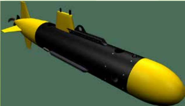
The SeaCat Hybrid is an example of an Autonomous Underwater Vehicle/Remotely Operated Vehicle that may be used to approach areas of interest and verify underwater munitions.
