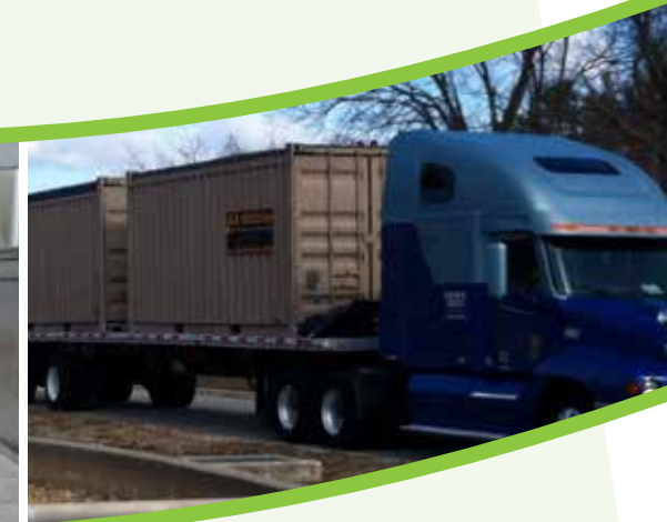
The NDCEE demonstrated a mobile, containerized wastewater treatment system at Fort Leonard Wood, assessing performance, energy use, and ease of mobilization and demobilization.
