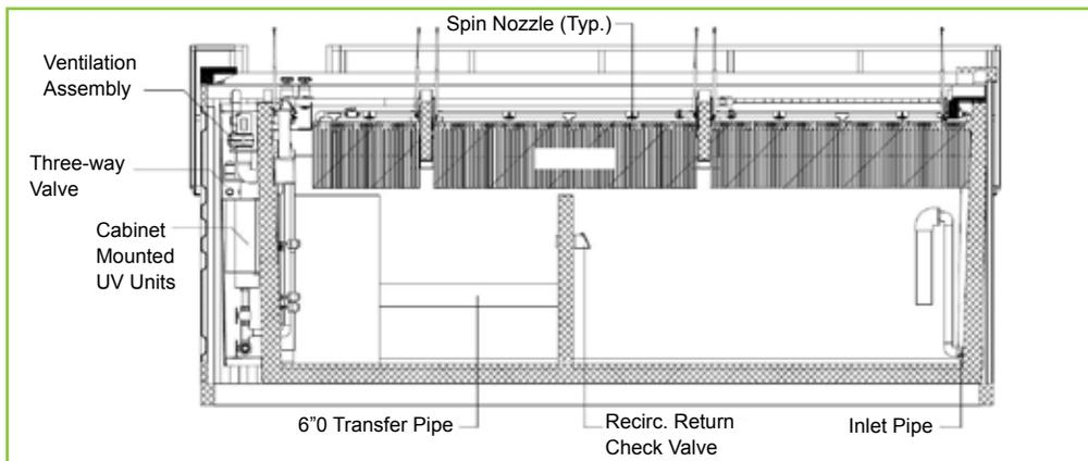
Diagram of secondary treatment unit with textile filters
