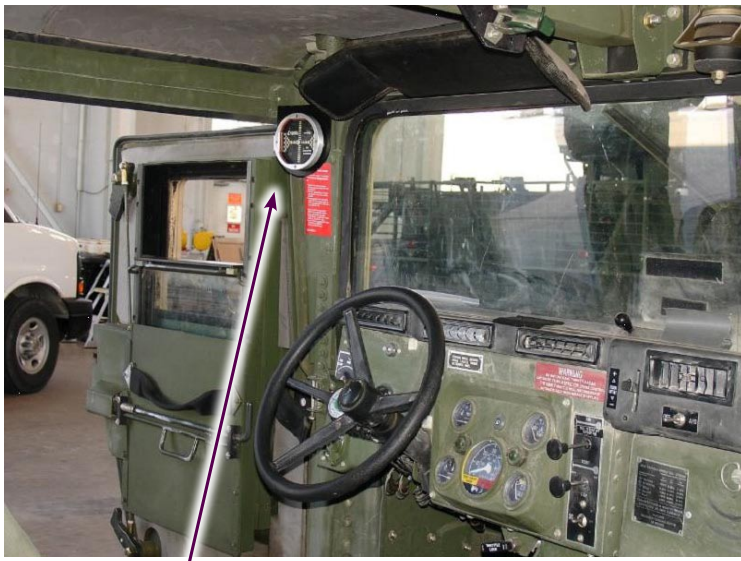
The rollover alert device was installed in the top left corner of the HMMWV cab where a driver could refer to it.
