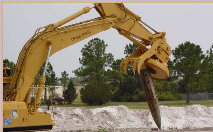
AFRL adapted the electromagnet to an Automated Ordnance Excavator (AOE) for this NDCEE demonstration.
