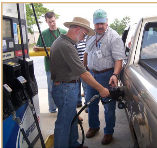
The dripless nozzle can reduce gasoline spillage during vehicle refueling, creating both EHS and cost benefits.
