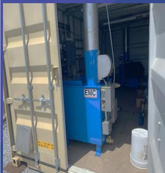
Pair of pilot scale thermal evaporators installed at the Silver Flag training site (Tyndall AFB)
