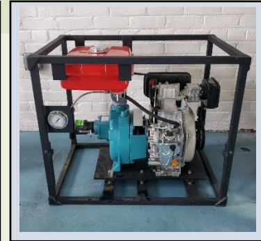
FEED PUMP SKID
