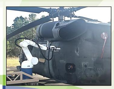
2019, TRL 5 AR3P CDP Configuration, UH-60L, dry engagements (engine/rotors static), approach from side, passed fuel to the aircraft.
