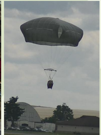
CAADS bundle equipped with a T-11 main parachute loaded on aircraft (left) and the bundle in flight under canopy (right)
