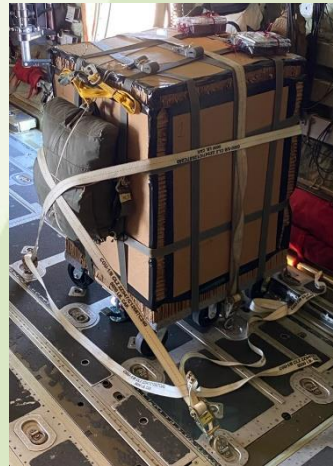
CAADS bundle equipped with a T-11 main parachute loaded on aircraft (left) and the bundle in flight under canopy (right)
