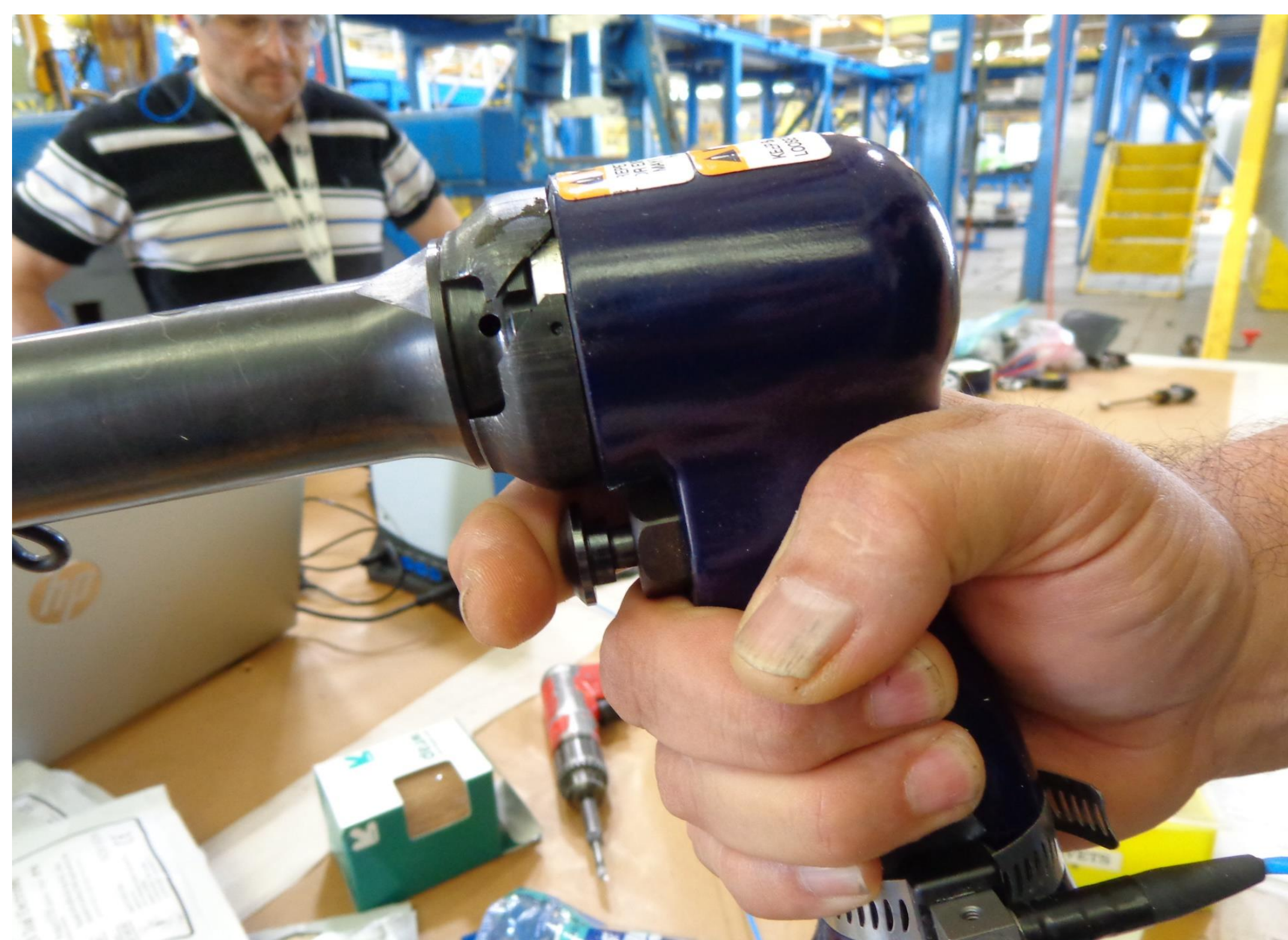
Figure 1. Honsa® HTOP-38 rivet hammer DCPH-A photo by John Pentikis
