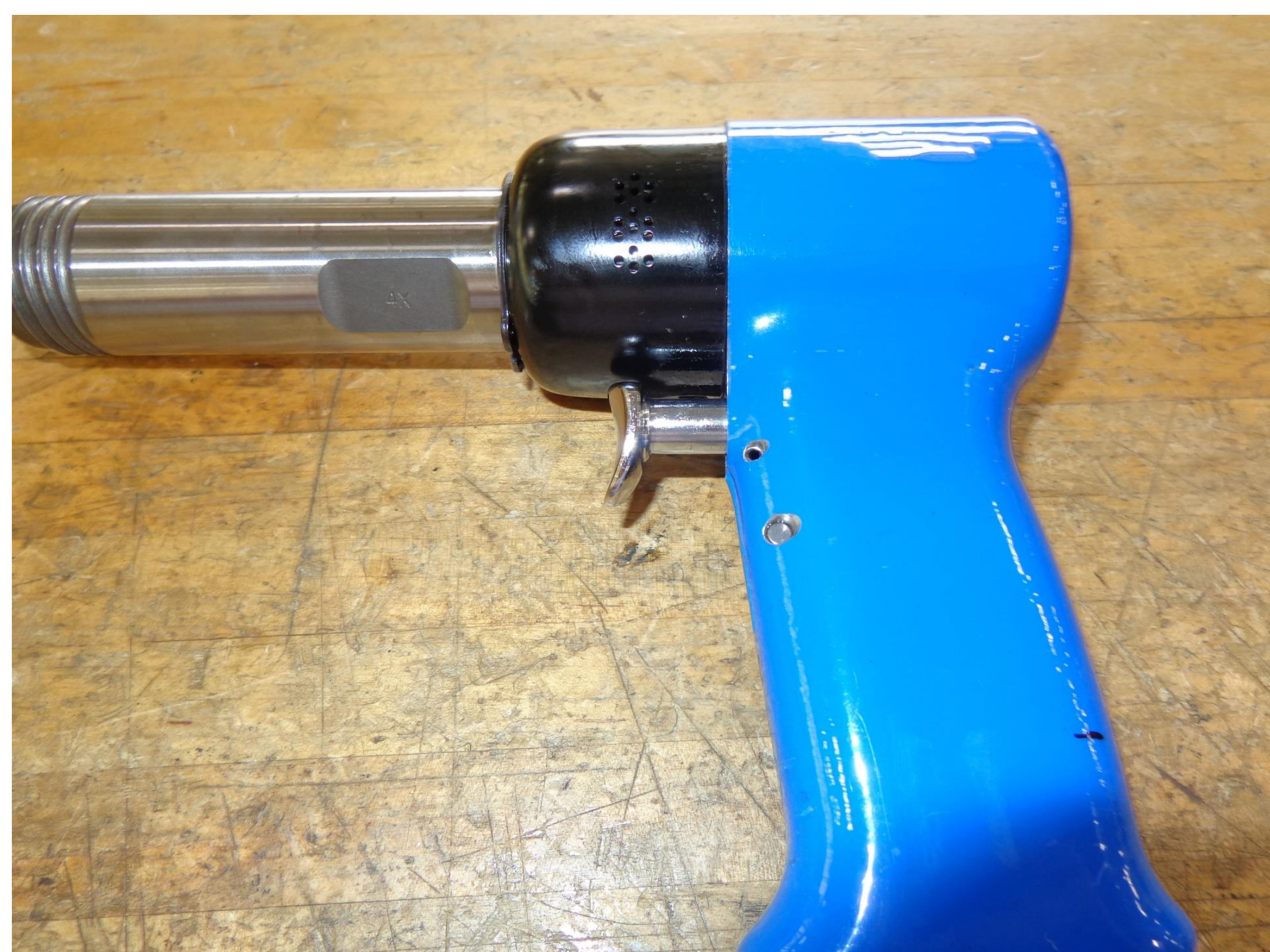
Figure 2. ATI® ATC rivet hammer DCPH-A photo by John Pentikis
