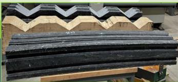
Recycled rubber/plastic railroad ties cut out by automated waterjet replacing wooden sweeps
