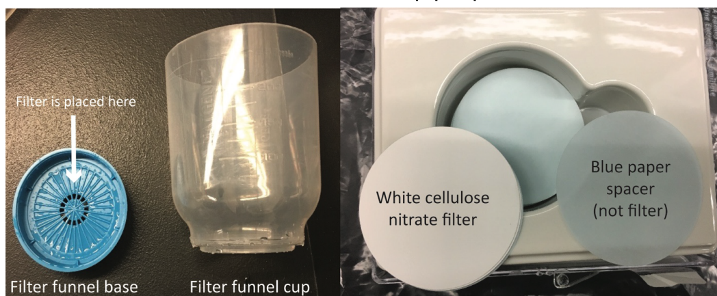
Figure 2. Example of the filter funnel components and how to differentiate the cellulose nitrate filters from the blue paper spacers.
