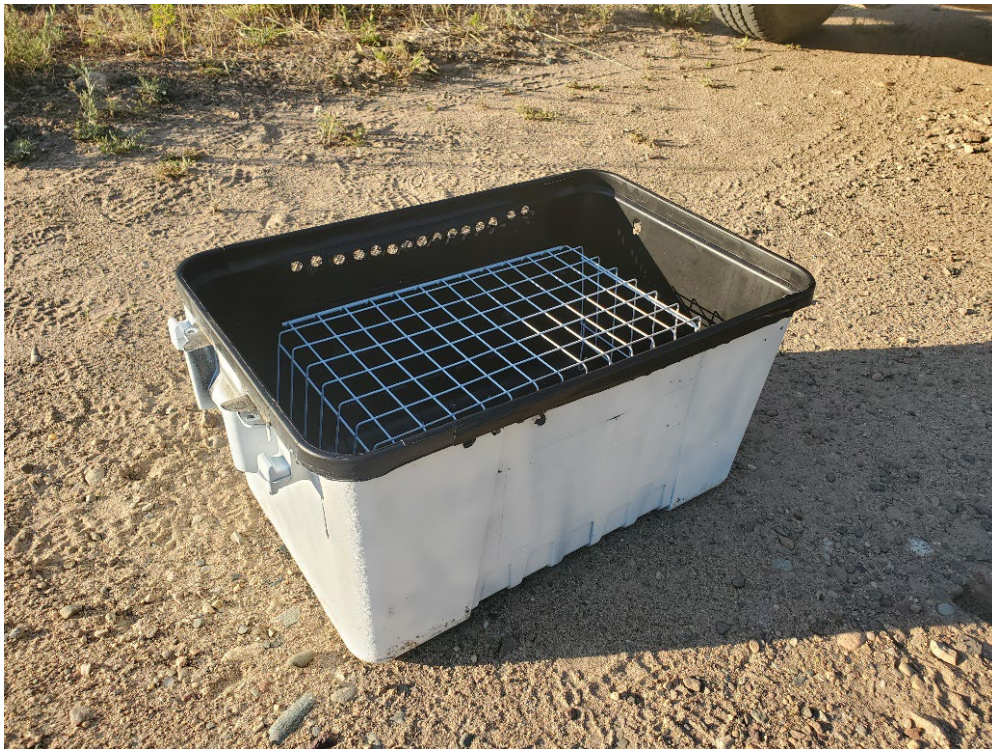
Figure 1. View inside of laptop storage tub. Air holes are visible near the top lip of the tub, and wire shelf allow airflow for the laptop to prevent overheating. External battery fits next to the wire shelf.
