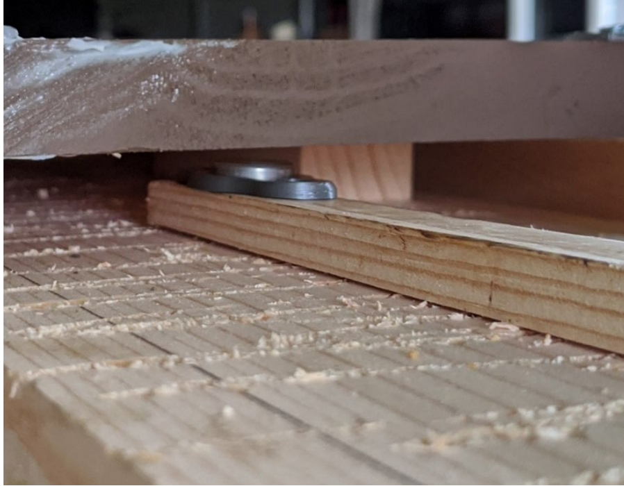
Figure 4. Visually inspect mounted iButtons to ensure that the iButton is not in contact with the outer shell (brown) of the rocket box.
