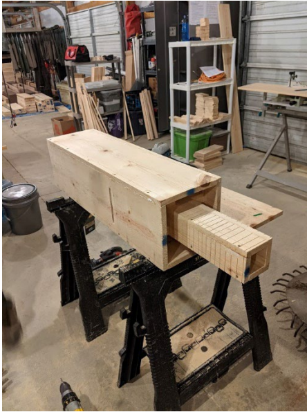
Figure 4. Single-chamber rocket box with vents on two sides used in Florida.
