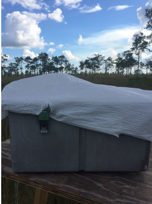
Figure 2. Solar shield over box with lure components.
