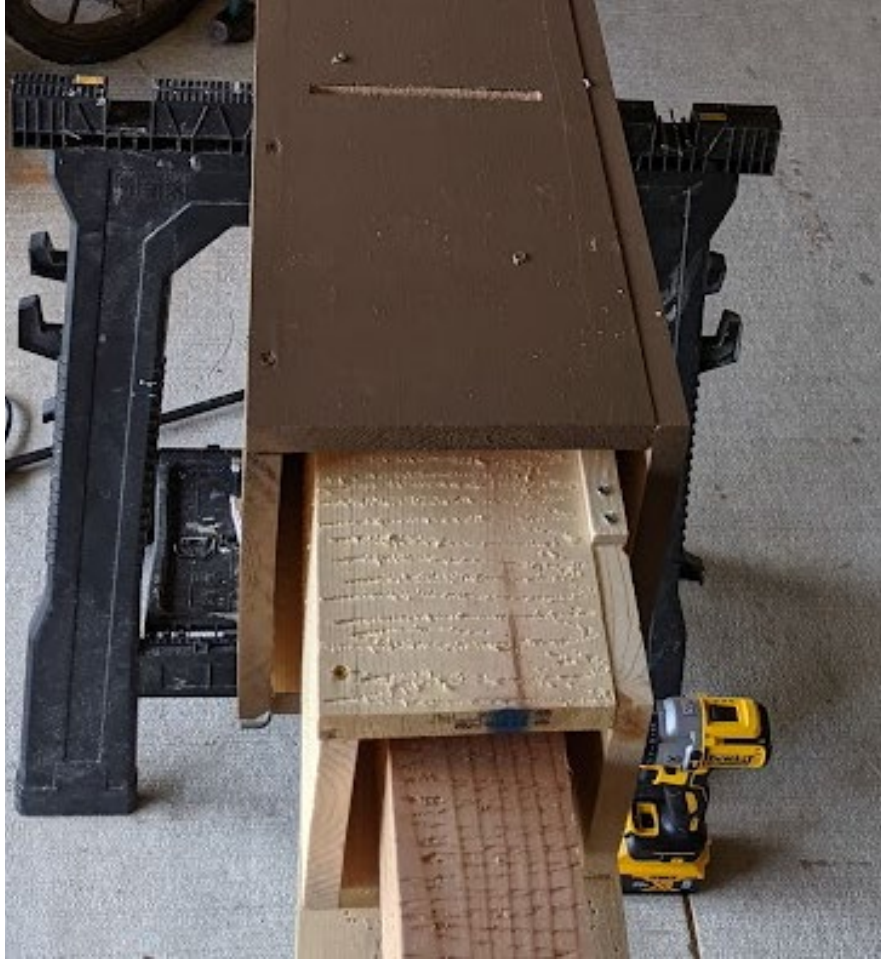
Figure 6. Example of an iButton stick inserted and anchored to the inner shell of a rocket box using two 3/4" #6 screws.
