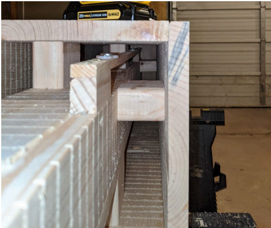
Figure 5. Example of iButton lath sticks mounted on raising spacers.
