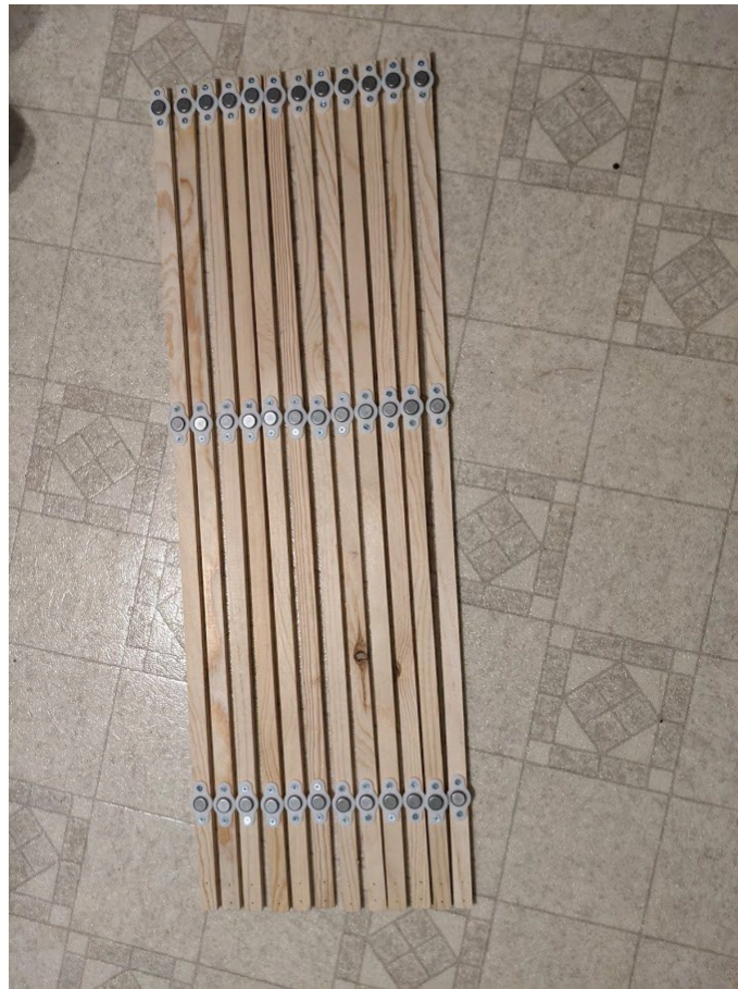
Figure 3. iButtons mounted to lath strips using 3D printed mounts.
