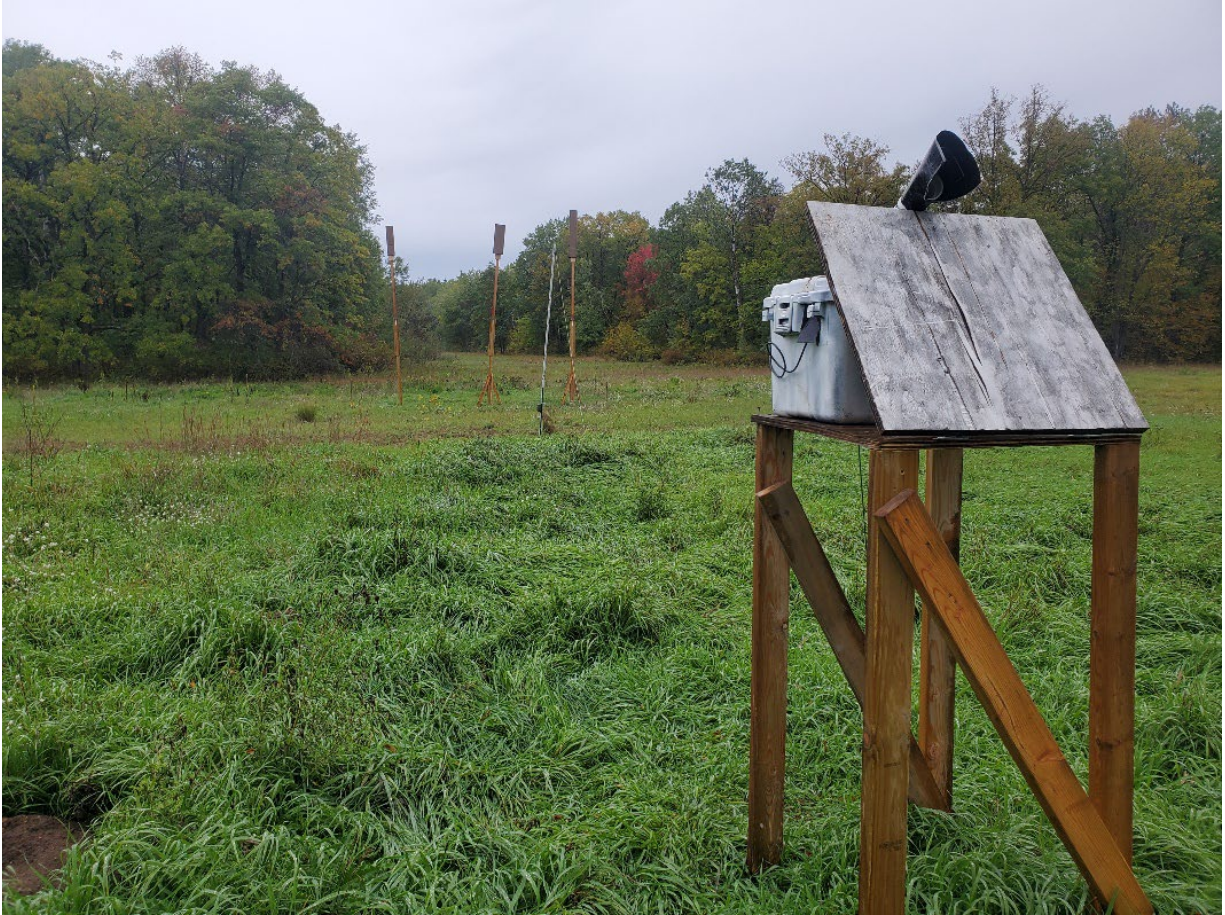
Figure 2. Complete lure set-up on the wooden stand. Lure speaker faces south, pointed away from the bat boxes and acoustic detector (pictured in the foreground). White tub houses and protects computer, battery, and cables. Lure speaker is housed in PVC pipe and dryer duct (not seen), while the black rain guard keeps water from entering speaker.
