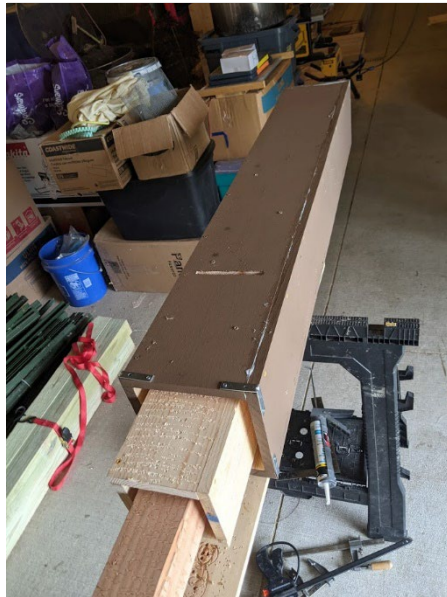
Figure 9. Two-chamber attic rocket box design used in Minnesota.
