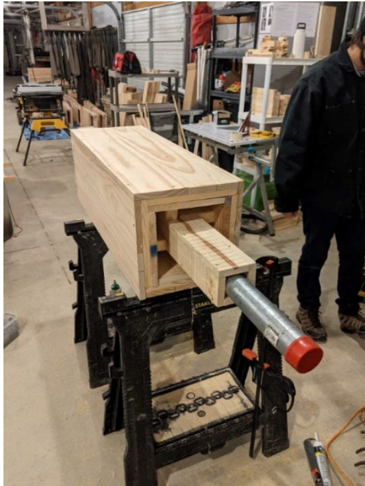
Figure 5. Single-chamber external water jacket box with no external vents used in Florida.
