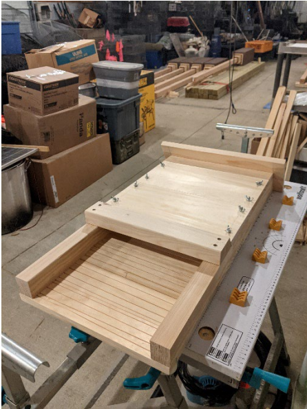
Figure 6. Single-chamber flat-faced box typically used for Florida bonneted bats.
