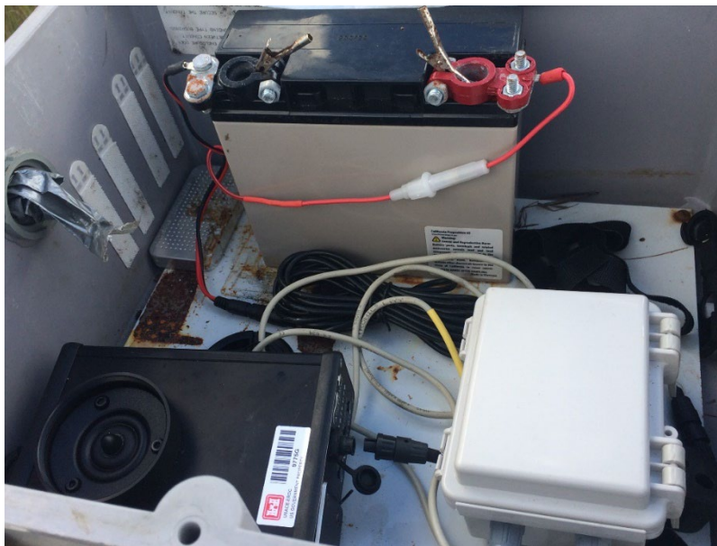
Figure 3. Inside of box with battery, timer, and lure device.
