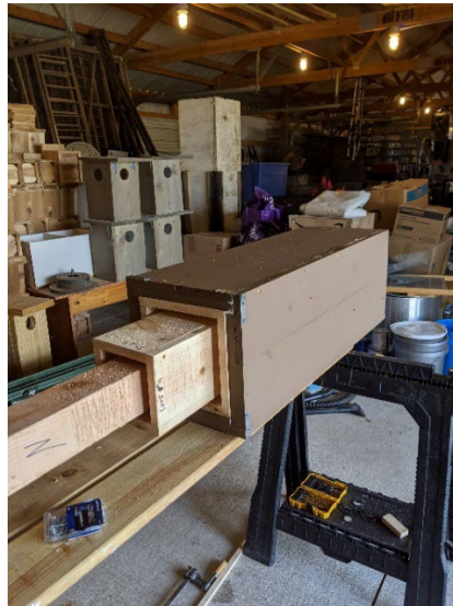
Figure 8. Two-chamber external water jacket rocket box design used in Minnesota.
