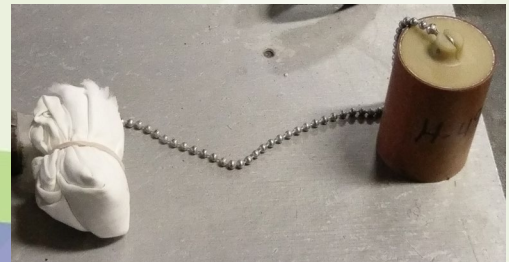
Flare composition pressed into flare with parachute mounted
