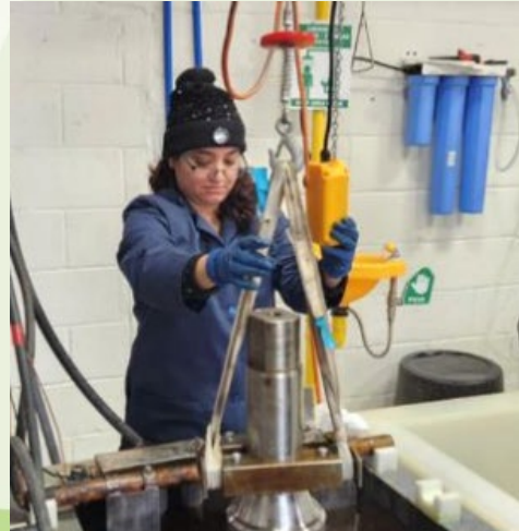
H-Max being applied to steel rollers which gave twice the wear resistance compared to hard chrome
