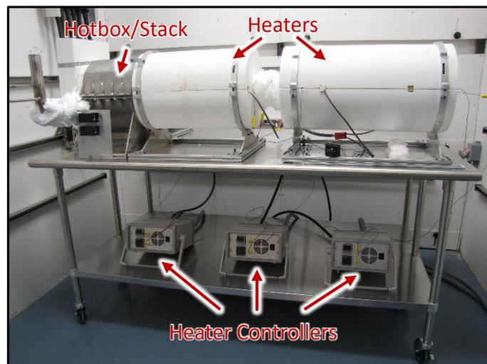
SOFC Stack Testing Apparatus
