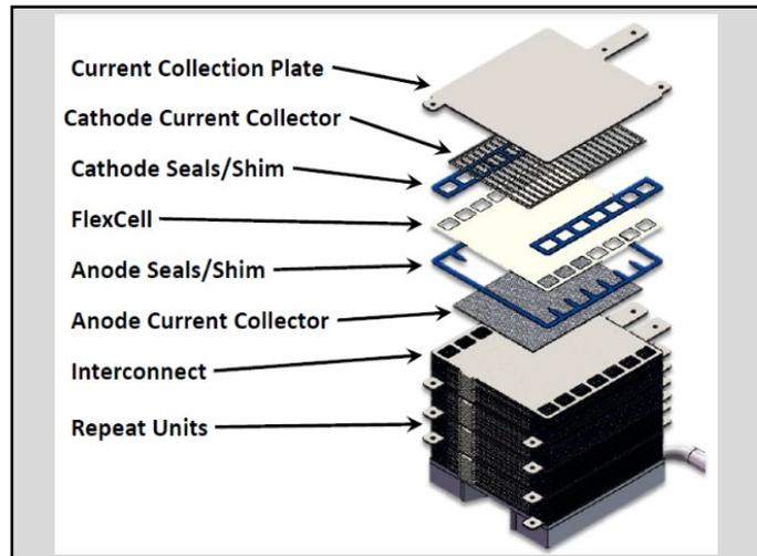
Expanded View of SOFC Stack
