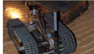
Radio-controlled robotic devices such as this allow caves to be surveyed with minimal impact or disturbance.
