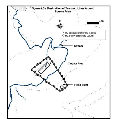
Figure 4.5b represents the source area bounded with closed sampling Transect Lines. The circles represent sampling segments and the black dots represent sampling segments where results were found to exceed the screening level. The dashed line represents the boundary of the source area after linear adaptive sampling.
