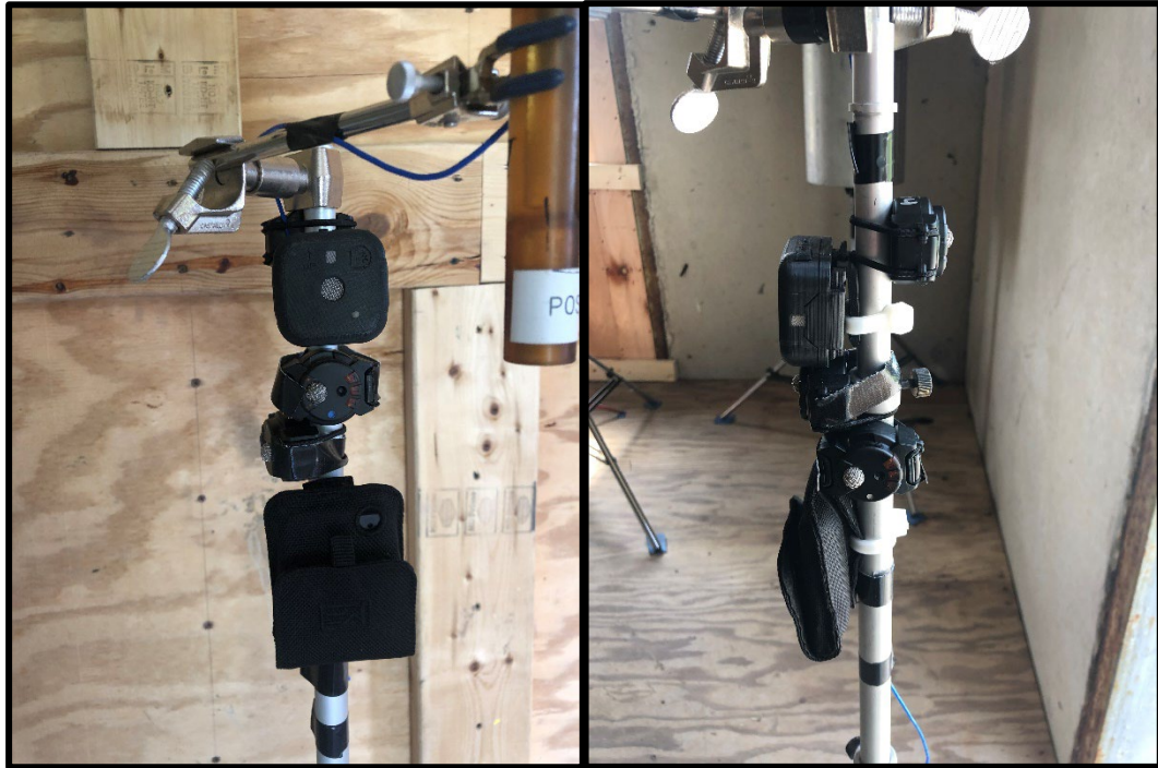
Figure 3. Blast Instrumentation Mounted on a Stake
