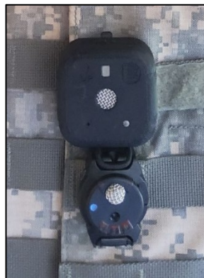
Figure C-1. L3 Applied Technologies Incorporated Blast Dosimeter (top) and a BlackBox Biometrics Gen7 Blast Gauge (bottom)
