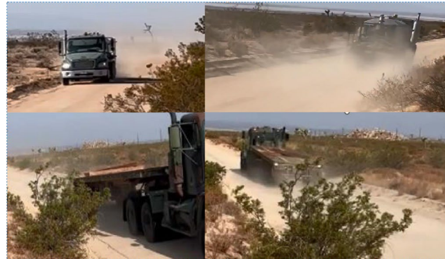
Edwards Air Force Base, Dust Generation at 35 mph Prior to Application (Top) and 6 Months After Application (Bottom)
