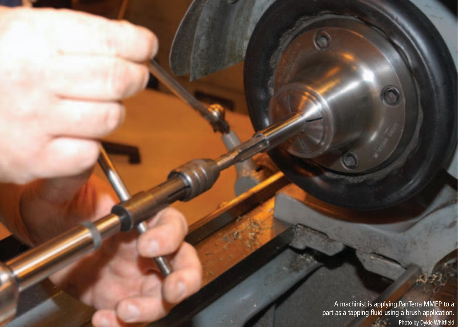
A machinist is applying PanTerra MMEP to a part as a tapping fluid using a brush application.
