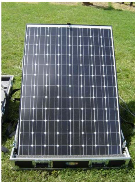
The Ground Renewable Expeditionary Energy System (GREENS) is powered by the sun. It is a 300-watt, photovoltaic/battery power system that provides continuous power to Marines in the field.
