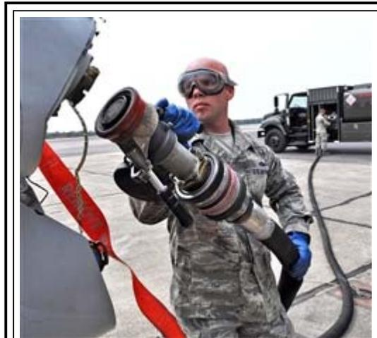
*Air Force Staff Sgt. Rusty Jones prepares to fuel an A-10C Thunderbolt II with a 50/50 blend of synthetic fuel and JP-8 at Eglin Air Force Base, Fla., March 25, 2010. The A-10 then flew the first flight of an aircraft powered solely by a biomass-derived jet fuel blend. U.S. Air Force photo by Samuel King Jr. (Click photo for screen-resolution image):[high-resolution image](#) available.*
