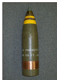
A NEW 5-INCH 38 CALIBER PROJECTILE (ABOVE). RECOVERED 5-INCH 38 CALIBER PROJECTILES (BELOW).
